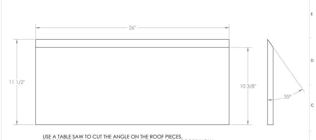
USE A TABLE SAW TO CUT THE ANGLE ON THE ROOF PIECES.
